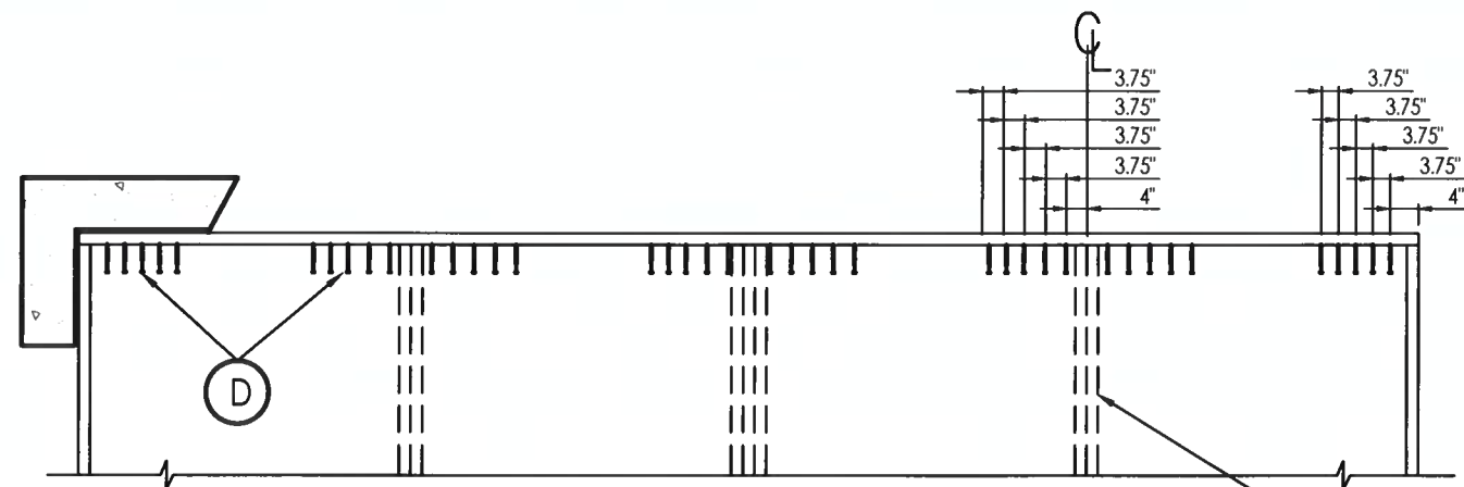
FRAME ANCHORING @ HEAD DP <= 80 PSF Max. shim space <= .625
